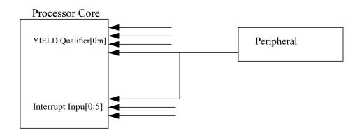
In more complex system configurations, incoming signals may be filtered and multiplexed by intermediary logic, configurable by software to map system signals to YIELD qualifiers as required by the application.
