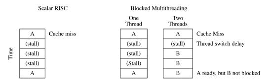
Because blocked multithreading changes threads less frequently, its implementation can be simplified. On the other hand, it is less "fair" in scheduling threads. A single thread can monopolize the processor for a long time if it is lucky enough to find all of its data in the cache.
